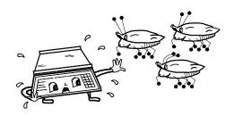
6.- PROTECT THE SCALE FROM INSECTS (MAINLY FROM ROACHES) THEY CAN SERIOUSLY DAMAGE THE ELECTRONIC COMPONENTS. USE SOLID PRODUCTS AGAINST ROACHES.
