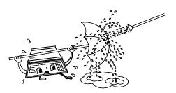
5.- "NEVER" WASH THE SCALE USING A FLOW OF WATER .THIS CAN DAMAGE THE ELECTRONIC COMPONENTS. FOR MORE INFORMATION READ "MAINTENANCE AND CLEANING" SECTION.
